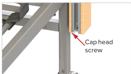
10.7 Cap head screw replaced
