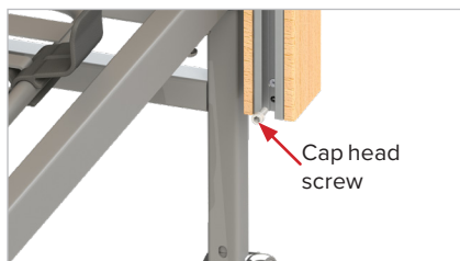
10.1 Cap head screw removed
